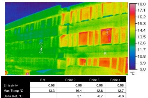
3. This image is of the same area as image no.2 but after the next section was refurbished. It can be seen that the main entrance and the top of the windows in the new section show the most heat loss.
