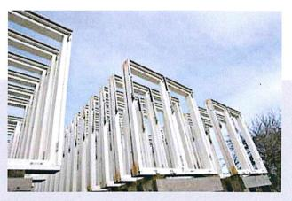
Window frames on a windswept hilltop. Our test department compares here the durability of different types of surface treatment.
