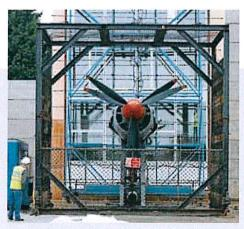
CWCT accredited. A 58m<sup>2</sup> large window screen tested for wind load. Part of the CWCT test includes an aircraft engine simulating very strong wind.
