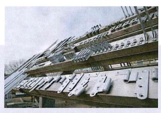
VELFAC R&D Department develops most of our ironmongery, so they are adapted specifically for each window system. The ironmongery are regularly tested both internally and at test institutes. Here are ironmongery exposed to salty Westcoast wind and weather as part of internal test.
