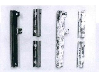
After the CCT test (CCT evaluation value 10 jf. EN/ISO 10289) all VELFAC brackets must still be without a trace of rust. The difference between a VELFAC corrosion protection (left) and corrosion protection for the industry's traditional demands are clear.
