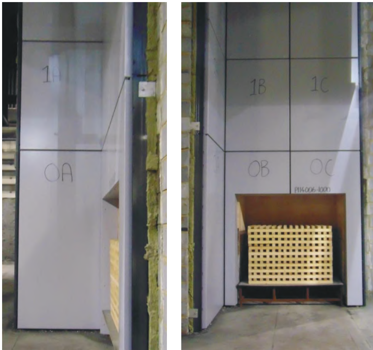
Figure 2. Photographs of completed build prior to test up to mid-height.
