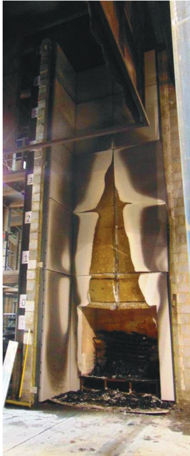
Figure 19. Full-height photograph of cladding system immediately after test.
